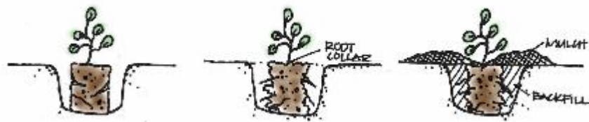
Figure 7: Container plant installation diagram
